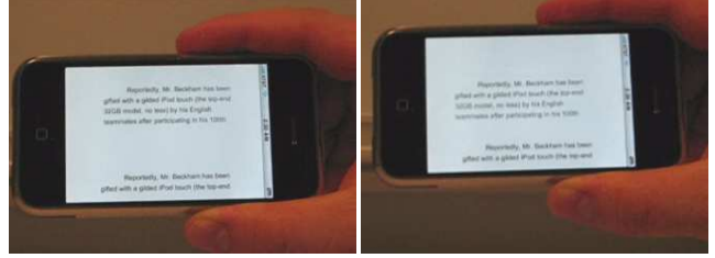
Figure 4: iPhone-based prototype with texts displayed for the user study. Only the first paragraph on the screen is stabilized by NoShake
