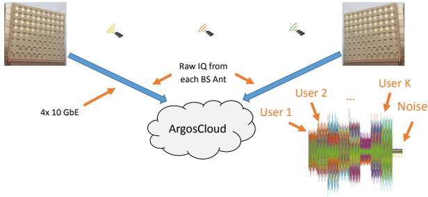
Fig. 5. Overview of the multi-cell channel measurement system design. At the beginning of each frame all base stations send a beacon to synchronize the users. Each user then sends orthogonal pilots, which every base station radio module records. At the end of the pilot phase, base-station radio modules report the raw pilot IQ samples to the ArgosCloud, which records them to an HDF5 file.
