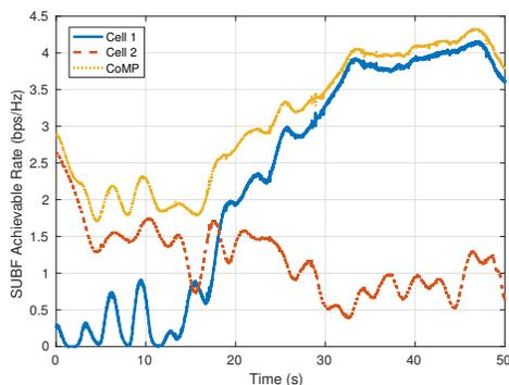
Fig. 7. Achievable rate of a user moving from one 10-antenna cell to another over time when be served by each cell individually as well as CoMP with coherent joint transmission, i.e., beamforming.
