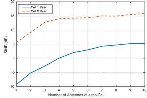
Fig. 6. SINR of users vs. number of base station antennas in two cells, each with one user. Increasing the number of base station antennas naturally reduces network interference through beamforming.
