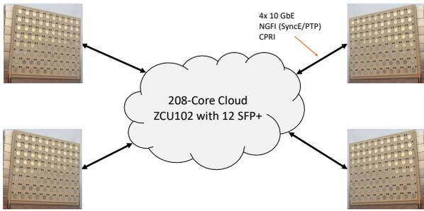
Fig. 4. ArgosNet logical architecture. Each base station has four single-mode 10 GbE fiber pairs connected to the 208-core ArgosCloud. In addition to commodity servers, the cloud has a 52-port 10 GbE switch and a Xilinx ZCU102 development kit for distributing NGFI (SyncE/PTP) or CPRI. The ZCU102 has four built-in SFP+ ports, and can be expanded to up to 20 SFP+ ports using FMC expansion cards.
