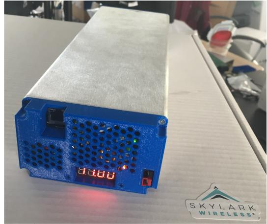
Fig. 2. ArgosMobile with integrated WiFi, GPS, and a 12-hour battery life.
