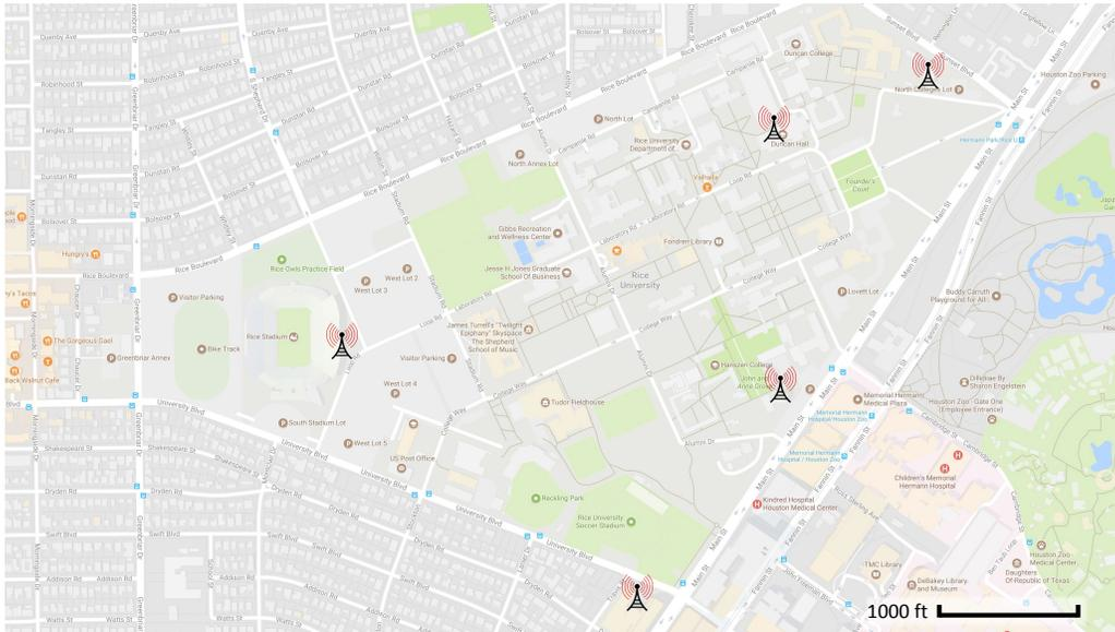
Fig. 3. ArgosNet base station locations. Each location has mounting, power, and direct fiber to ArgosCloud. All locations are outdoor sites except for Duncan Hall *top middle*, which is our indoor lab environment.
